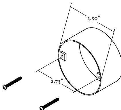
The backplates on this fixture are 4 inches in diameter and are made of solid metal (not pressed) so junction boxes must be flush with wall surface.
