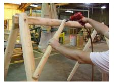
11. Stand frame upright and tighten nuts on 7 ½" machine bolts enough to allow frame to stand freely.
