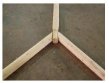
9. Position top pole on ground with swing hooks facing downward. Position legs and install 7 ½" machine bolt and washer through legs and top pole, install a second washer and nut. *Finger tighten only at this point*.
