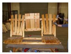
2. Position pre-assembled tabletop, with underlay tenon, in hole on side of seat back (as shown). Repeat this process for remaining seat. Use rubber mallet to fully insert all seat back tenons into seat bottom.
