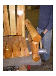
6. Attach both swing arm assemblies to swing seat. Align the two tenoned ends of swing seat with the two holes in the swing arm assembly. Tap arms into place using rubber mallet.
