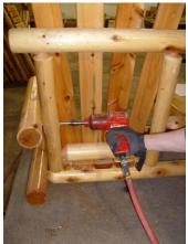
7. With a 3 3/8" lag bolt and 1/4" washer, secure seat back to the swing arm as shown. Repeat this process for the opposite side. Using 2" screws capture all tenon joints as shown.
