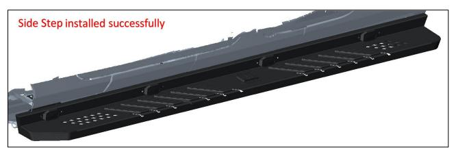
**Step 6:** Adjust the balance of the Side Step and the car side, and tighten the corresponding bolts.
