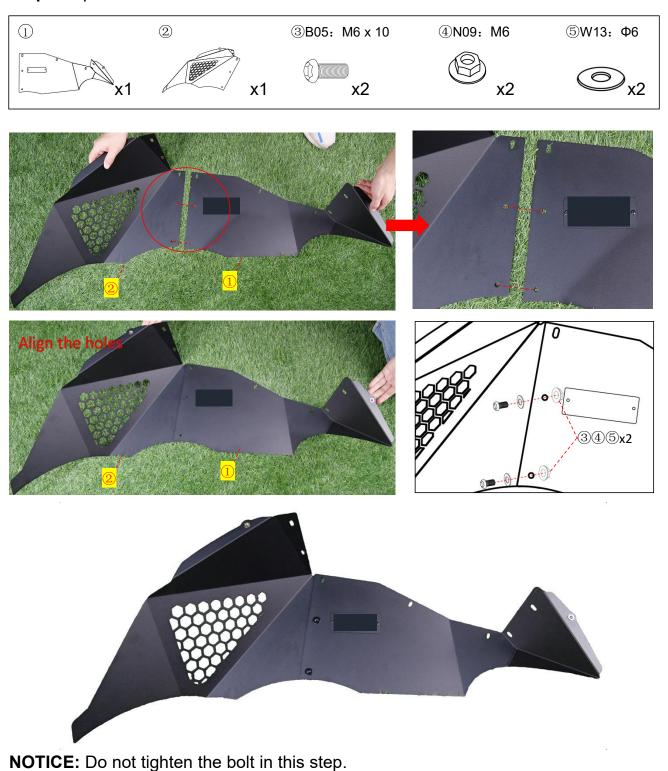
**Step 3:** Splice the rear inner fender flares.
