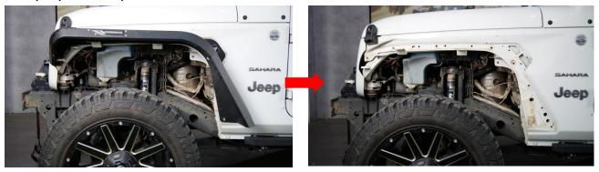
**Step 3:** Install the front inner fender flares 2.
