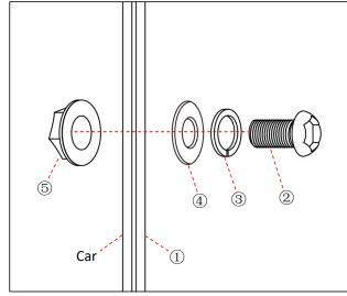
**Step 4:** Install the front inner fender flares 1.
