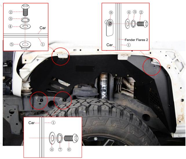
Step 5: Install the front inner fender flares 3 or front inner fender flares 4.
