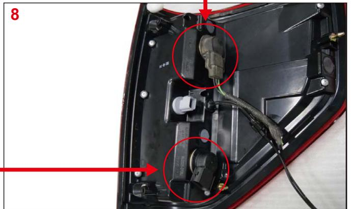
9. Place the resistor in a safe location in the housing, and connect the resistor. (First, use the 7.5HM resistor. If there is a flicker, please replace the 7.5HM resistor with the 4.0HM resistor.)
