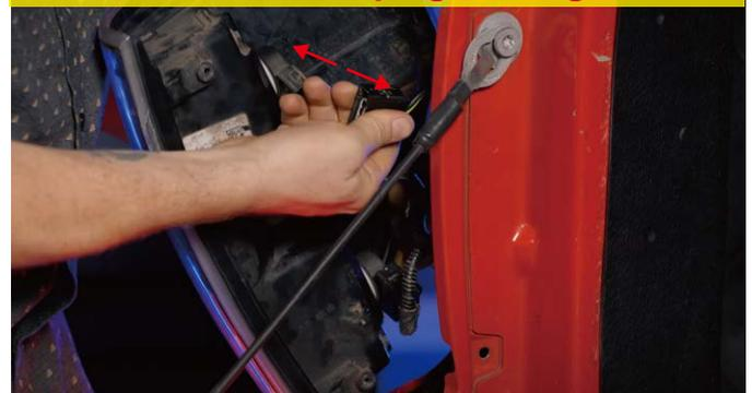
**Grab either one of the black connectors and white connector on the truck and plug them in the connector of the new taillight.**
