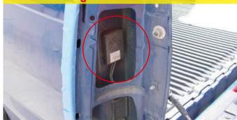
8. Connect the pigtails to the stock sockets.
