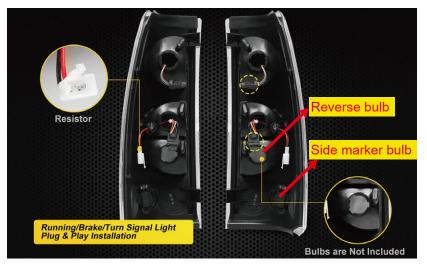
7. Place the resistor in a safe location in the housing.
