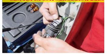
9. Connect the resistor to the taillight housing.
