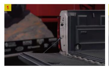
2. Open the tail gate and locate the two screw and remove them.
