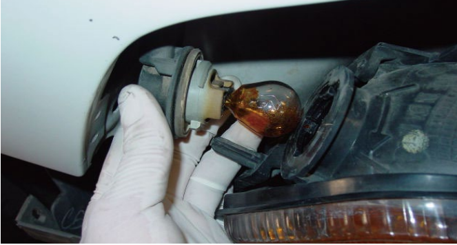
7. Twist off the corner light from the headlight.
