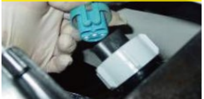
10. Put in the new light and plug in the headlight harness.
