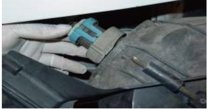
8. Unplug the headlight bulb from the housing.
