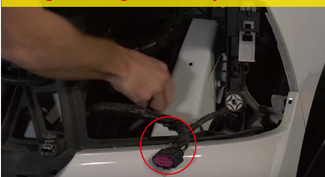
9. Plug the headlight with factory connector.
