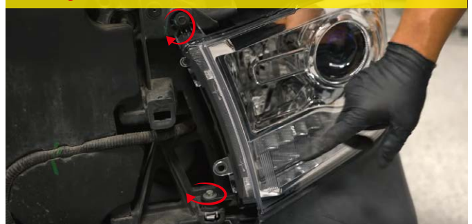
10. Put the headlight on the car and secure it with factory 10mm bolts.
