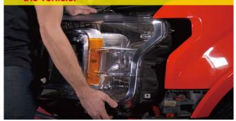
Remove the high beam bulb, low beam bulb and side marker bulb, take them onto the new headlight.
