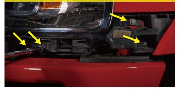
12. Remove two bolts on the top of the headlight.
