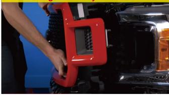
11. Remove the single eight millimeter bolt from the front, the rest of the bolts are ten millimeter.
