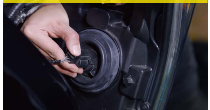
12. Connect all the factory harness plugs.
