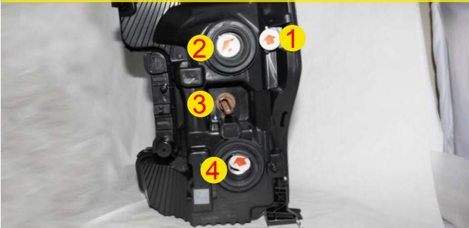
11. Put all the factory bulbs & sockets in the new headlight (except Turn Signal).
