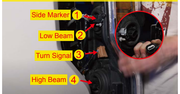
10. Disconnect four factory plugs.
