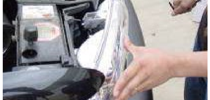
12. Put the headlight back into the housing and use the pins to lock in the headlight.
