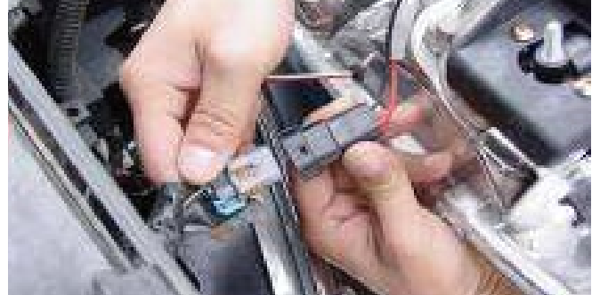
10. Connect the headlight plugs into the new headlight.
