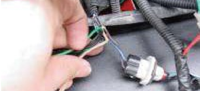
9. Splice the black(-) and brown(+) parking light to the new headlight. Red (+) wire to brown and black(-) to black.
