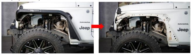
Step 3: Splice the front inner fender flares.
