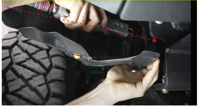
14. Cutting inner fender liner.
