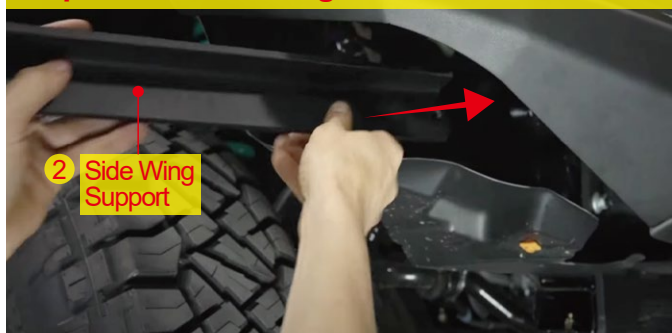
13. Install the wings to adjust the appropriate position for cutting the fender liner.
