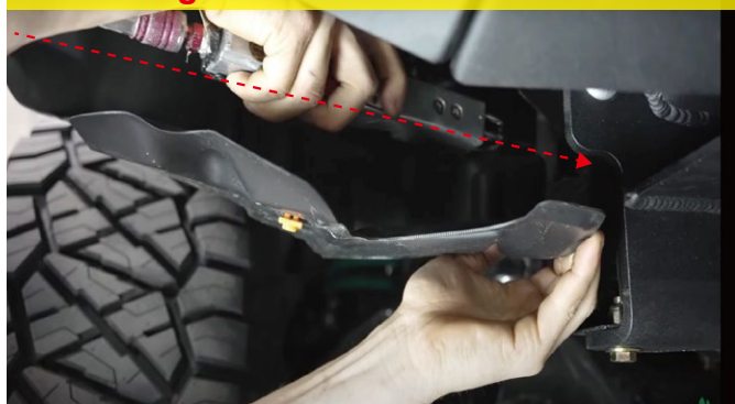
14. Cutting inner fender liner.
