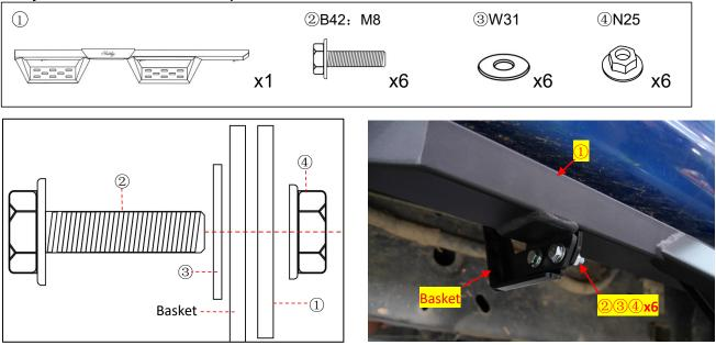
**NOTICE:** Do not tighten the bolts in this step.
