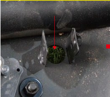
Radar probe install hole
