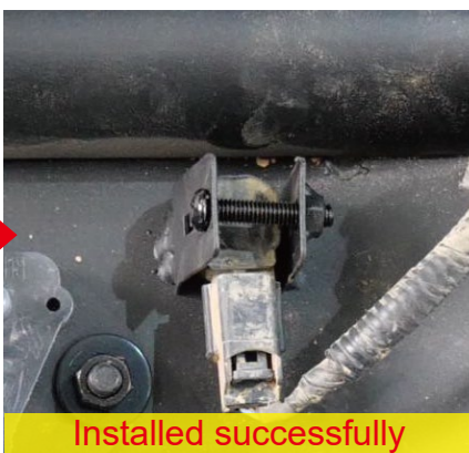
Plates must be clamp the radar probe
