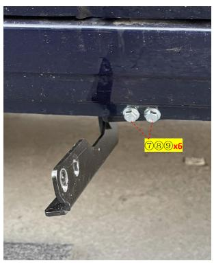
**NOTICE:** Please install the Original Bolts aligned with the Bracket holes according to the bottom of the car. Do not tighten the Bolts.
