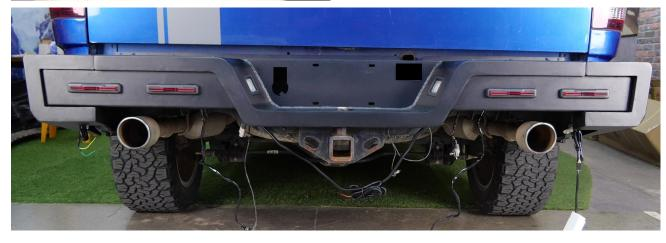
Step 7: Connect the bumper brake light wiring.
