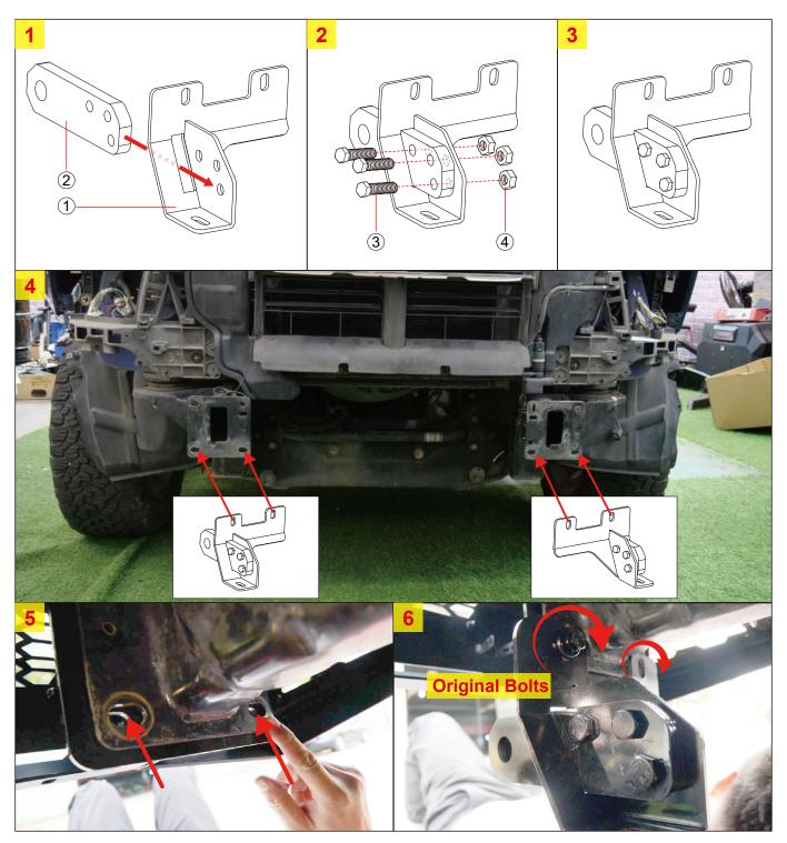
**Step 3:** Install the Winch Bracket.
