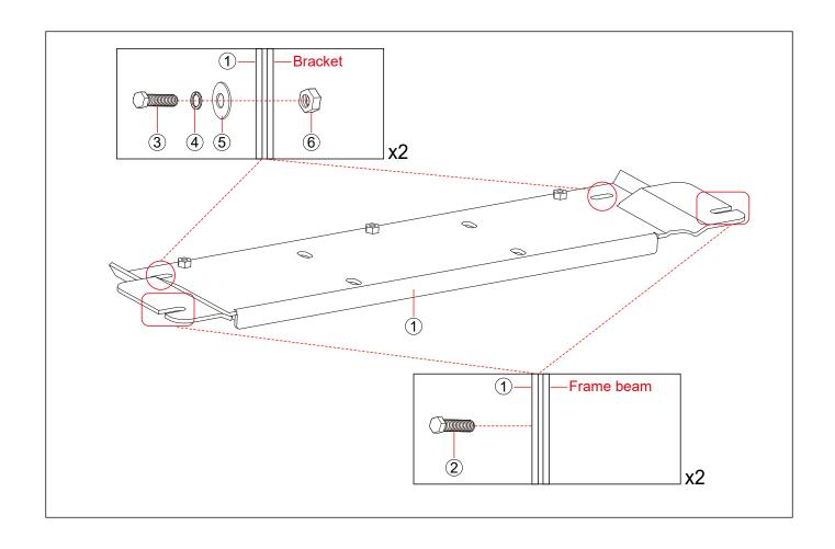
Step 4: Install the Skid Plate.
