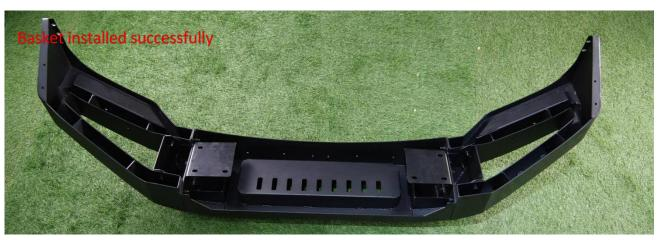
**Step 4:** Install the left and right plates and tighten the bolts.
