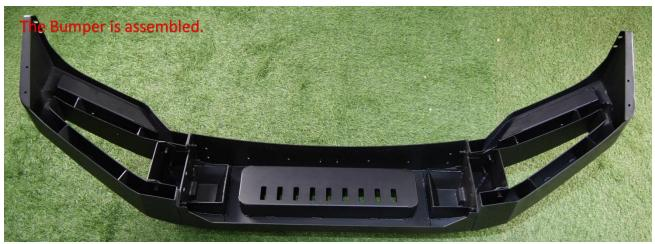
Note: Align of the Bumper and tighten the bolts.
