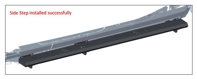
**Step 6:** Adjust the balance of the Side Step and the car side, and tighten the corresponding bolts.
