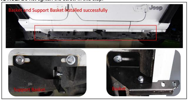
Step 7: Tighten the bolts fixed between the Support Basket and the car body.
