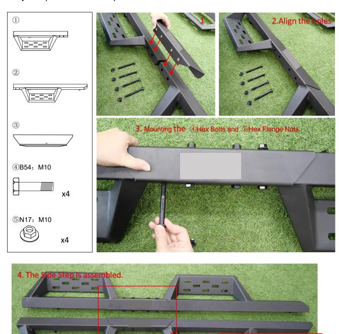
**NOTICE:** Before installing the Side Step on to the car, please ensure that the connecting bolts on the Side Step are all tightened.
