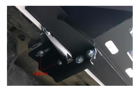
**Step 10:** Adjust the balance of the pedal to the ground and tighten the corresponding bolts.
