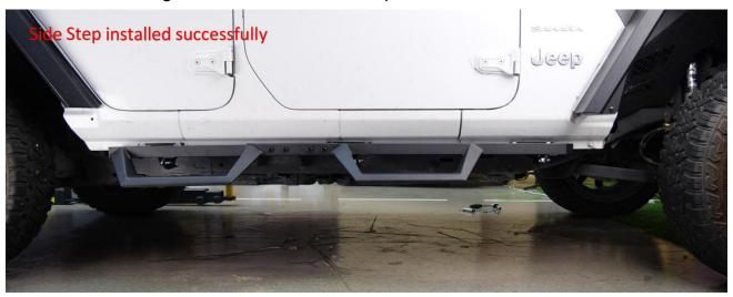
**Step 9:** Adjust the balance of the Side Step and the car side, and tighten the corresponding bolts.
