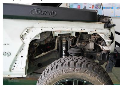
Step 3: Install the front fender flares and tighten the bolts.
