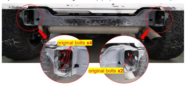
**NOTICE:** The car shown above has 6 original bolts, but other versions may have 2 bolts on the left and right sides, a total of 4 original car bolts.
