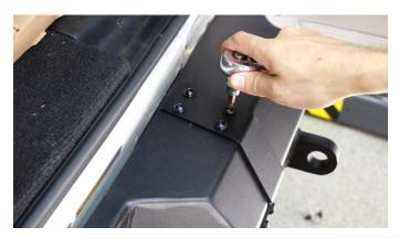
Step 8: Install the Tow Trailer Hitch Receiver.
