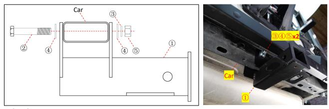
**NOTICE:** Do not tighten the screw in this step.
