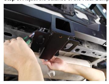
**Tips:** Use a stretch ruler to measure and balance the left and right sides of the Rear Bumper. Please ensure that the bumper has the same distance to the ground on both sides.
