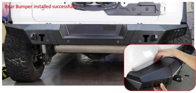
**Step 7:** Tighten all the connecting bolts on the Rear Bumper.
