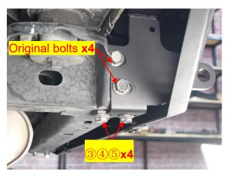
**NOTICE:** Do not tighten the bolts in this step.
