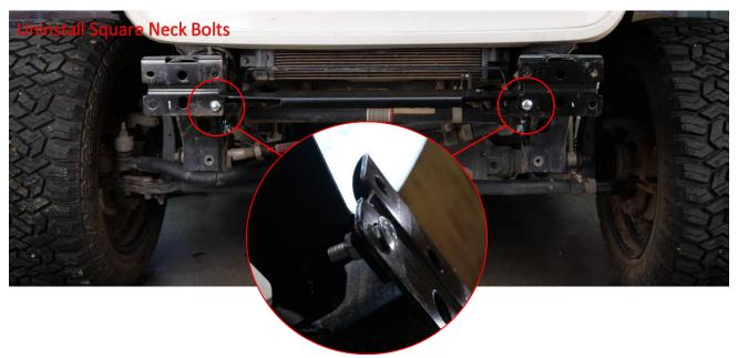
**Note:** The Bolt is only used to fix the Winch Bracket, and it is convenient to install the two mounting holes under the winch bracket. Please Keep it and use it in the next step.
