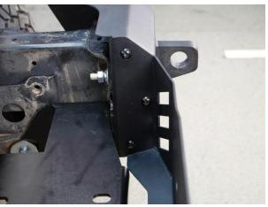
**Note:** Align of the Mid Bumper and Left/Right Bumper. Tighten the bolts of the Left/Right Bumper(**Step 4**) at the first, then tighten the bolts of the Mid Bumper.
