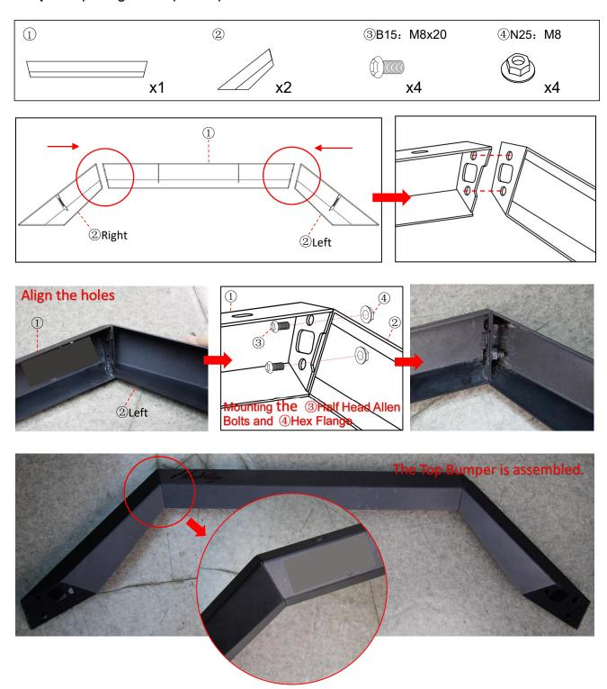
**Note:** Align of the Top Bumper and tighten the bolts.
