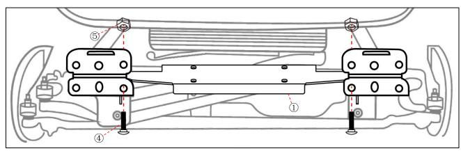
**Note:** Please mounting the corresponding bolts at the first. Do not tighten the bolt in this step. JK model do not need to use the ③Plate.
