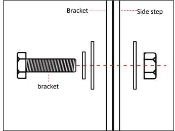
**Step 6:** Adjust the balance of the Side Step and the car side, and tighten the corresponding bolts.
