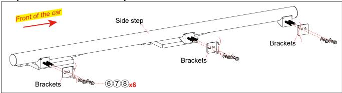
**Step 5:** Adjust the balance of the Side Step and the car side, and tighten the corresponding bolts.
