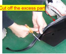
H-Rubber Strip Installed Successfully
