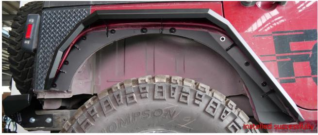
**Step 7:** Installation of a rear fender flares is complete. Please do periodic inspections of the fender flares to make sure that all hardware is secure and tight.
