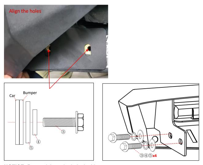
**NOTICE:** Do not tighten the bolts in this step.
