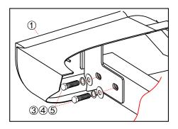
**Step 5:** Adjust the balance of the Rear Bumper and the car side and tighten the bolts.
