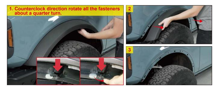
**Step 3:** Remove the original Rear Fender Flares.
