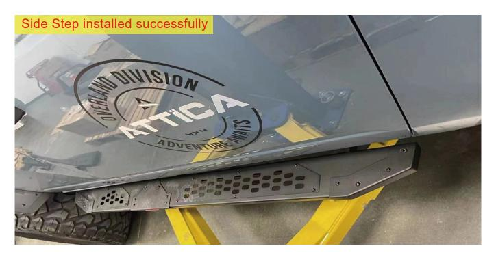
**Step 4:** Adjust the balance of the Side Step and the car side, and tighten the corresponding bolts.
