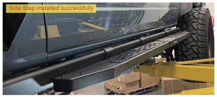
**Step 4:** Adjust the balance of the Side Step and the car side, and tighten the corresponding bolts.
