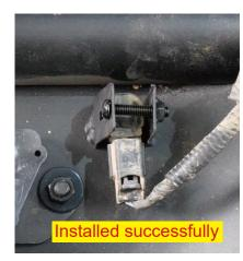
**Step 5:** Install the bumper and tighten the bolts.
