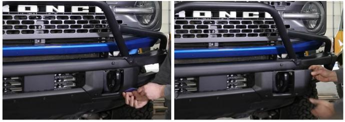
7.2: Use a 15mm socket to remove the three bolts holding the bumper in on each side. Be careful because they are the only things holding the bumper in place. Do not fully remove them until you are ready to pull the bumper off.
