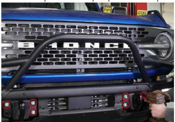
7.3: With the bumper off of the vehicle, use a 10mm socket to remove the small bolt in the middle of each of the metal brackets and remove metal brackdts.
