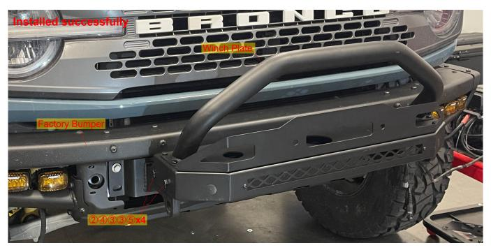
7.5: Install the vehicle bumper and Bracket 2.
