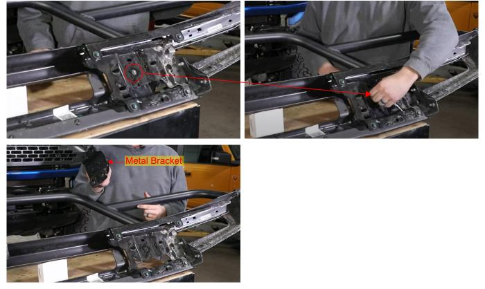
7.4: Install the vehicle bumper and Bracket 1.
