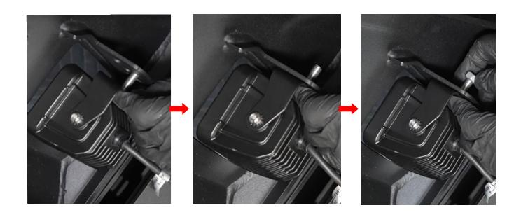
Step 5: Install the Winch Plate in the car.
