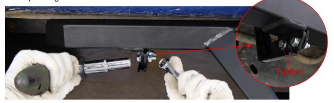
**Step 8:** Adjust the balance of the pedal to the ground and tighten the corresponding bolts.
