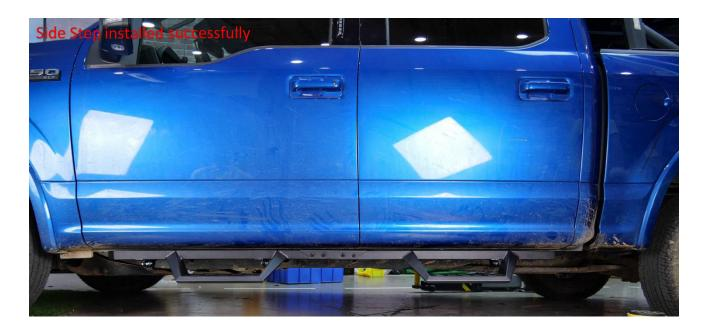
**Step 7:** Adjust the balance of the Side Step and the car side, and tighten the corresponding bolts.
