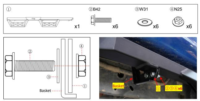
**NOTICE:** Do not tighten the screw in this step.
