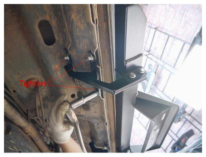
**Step 9:** Installation of a Side Step is complete. Please do periodic inspections of the Side Step to make sure that all hardware is secure and tight.
