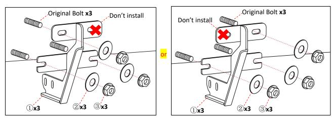
**NOTICE:** Please install the Original Bolts aligned with the Bracket holes according to the bottom of the car. Do not tighten the Bolts.
