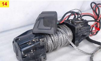
**Step 9:** Remove this top cover there are four Phillips head screws that come out and disconnet the plug. (figure15~16)
