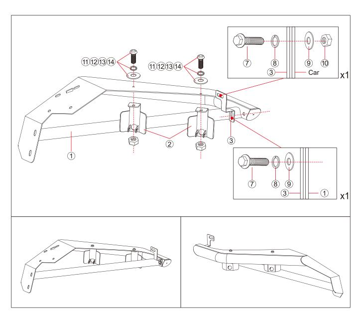
Step 3: Install the 4 Inch Ledlight.
