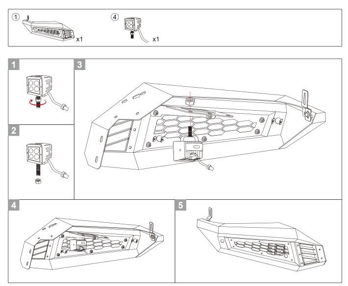
You can connect the 4inch Led light lights wiring harness to the headlight DRLs or fog light wiring. but my suggestion is to connect to the fog lights for on/off control!
