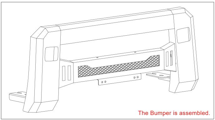
**Note:** Align of the Bumper and tighten the bolts.
