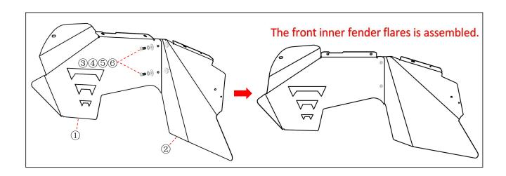
Step 4: Install the front inner fender flares.
