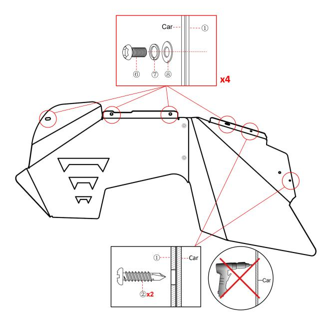
Step 5: Tighten all the bolts and nuts.
