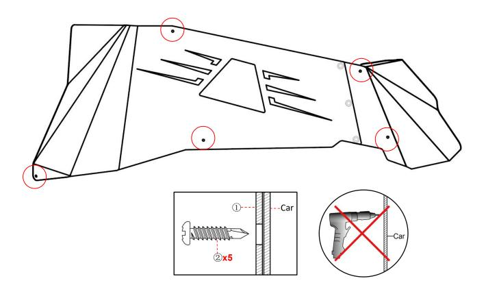
**Step 5:** Tighten all the bolts and nuts.
