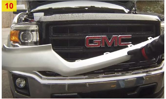
9. Loosen tab to remove front bumper trim more easily.
