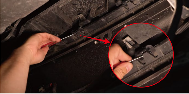
9. Loosen tab to remove front bumper trim more easily.
