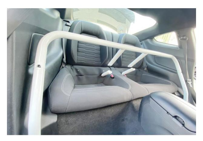
Once the side support bars are attached to the vehicle, you can now attach the main bar to the side support arms. It should look like the image above. Do not tighten the bolts down until both side bars are attached. Once attached you can tighten them down.
