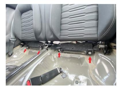
Attach the shortest support bar to the inner bolt but do not tighten down the bolt all the way yet so you can adjust it again later. Make sure the groove is facing upwards. There's no difference between each side of the support bar.
