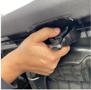
Remove the child seat anchors from both sides but keep the bolts as you will be re-using those later.
