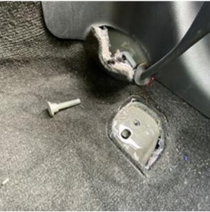
Grab the medium length side support bar. To determine which side is which, the bottom bracket should be facing toward the wall and the groove should be facing toward the front of the car. (see photo)
