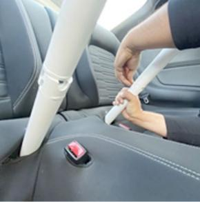
Next, line up the center support bars and tighten with those two bolts.
