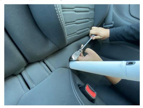
Once the main bar is attached to the center and side support bars you can now tighten down all the bolts. You can reach the center bolt mounts through the seat cushion to tighten it down to torque specs. Do the same for the side support bar bolt.
