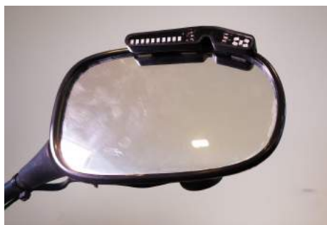
Correctly installed Alert Indicator
