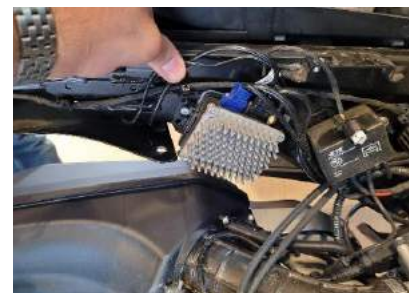
BMW C400GT - unit is placed between the frame and the under-seat storage
