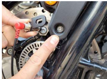
Fender bolt used to position the speed sensor next to disc bolt
