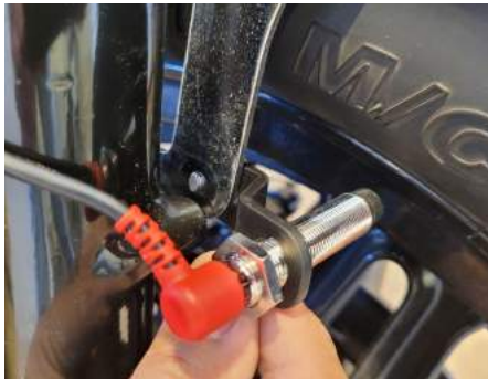
Fender bolt used to position the speed sensor next to wheel rim
