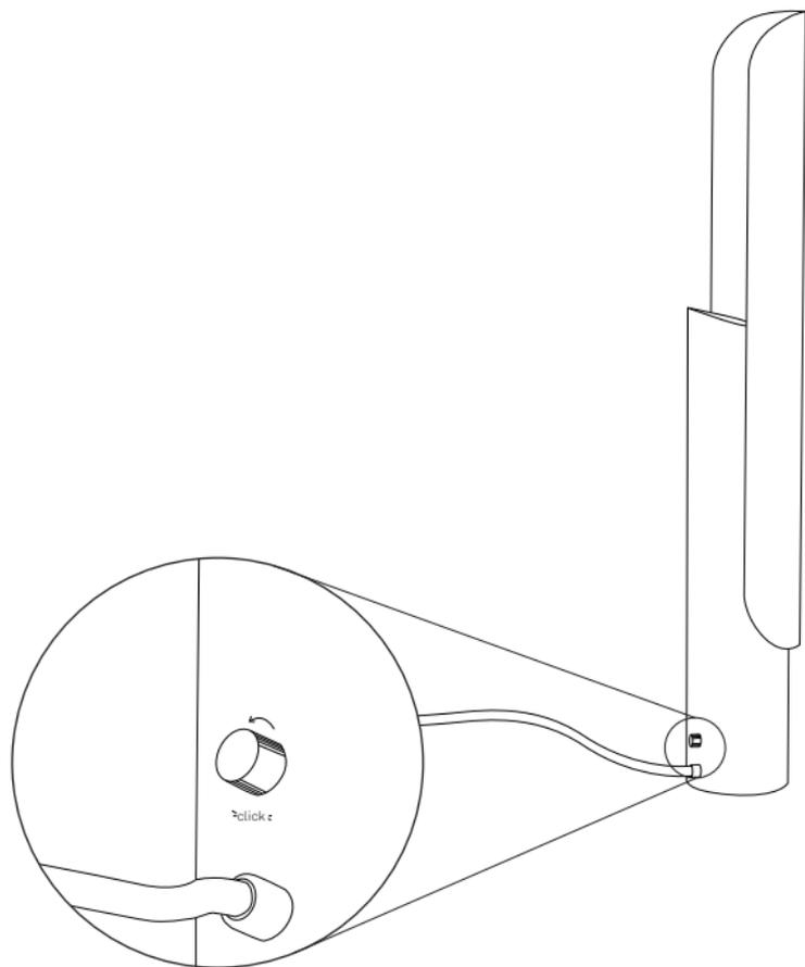
Start by unpacking the T-Lamp. There are no bulbs to screw in as an LED is already in place in the body of the Lamp. Plug the Lamp in and use the dimmer to choose the intensity of the light or to turn it off completely.
