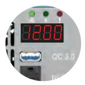
2.When the "ightharpoonup" indicator light is on, it indicates that the output power is being displayed.
