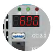
3.When the " $\mathbf{I}$ " indicator light is on, it indicates that the fault code is being displayed.
