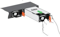
CAUTION: When inserting the PSU, do not use unnecessary force. Doing so can damage the connectors on the back of the PSU and on the midplane.
