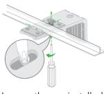
Loosen the pre-installed screw on the T-bracket so that the locking plate on the T-bracket can slide. Then secure the T-bracket to the T-bar and tighten the screw.
